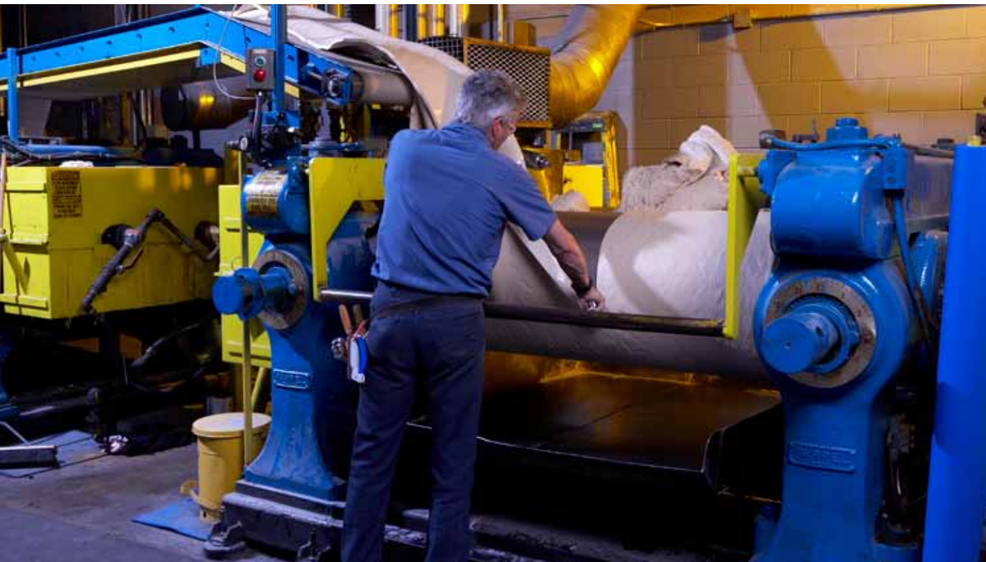
Protective linings warming mill
