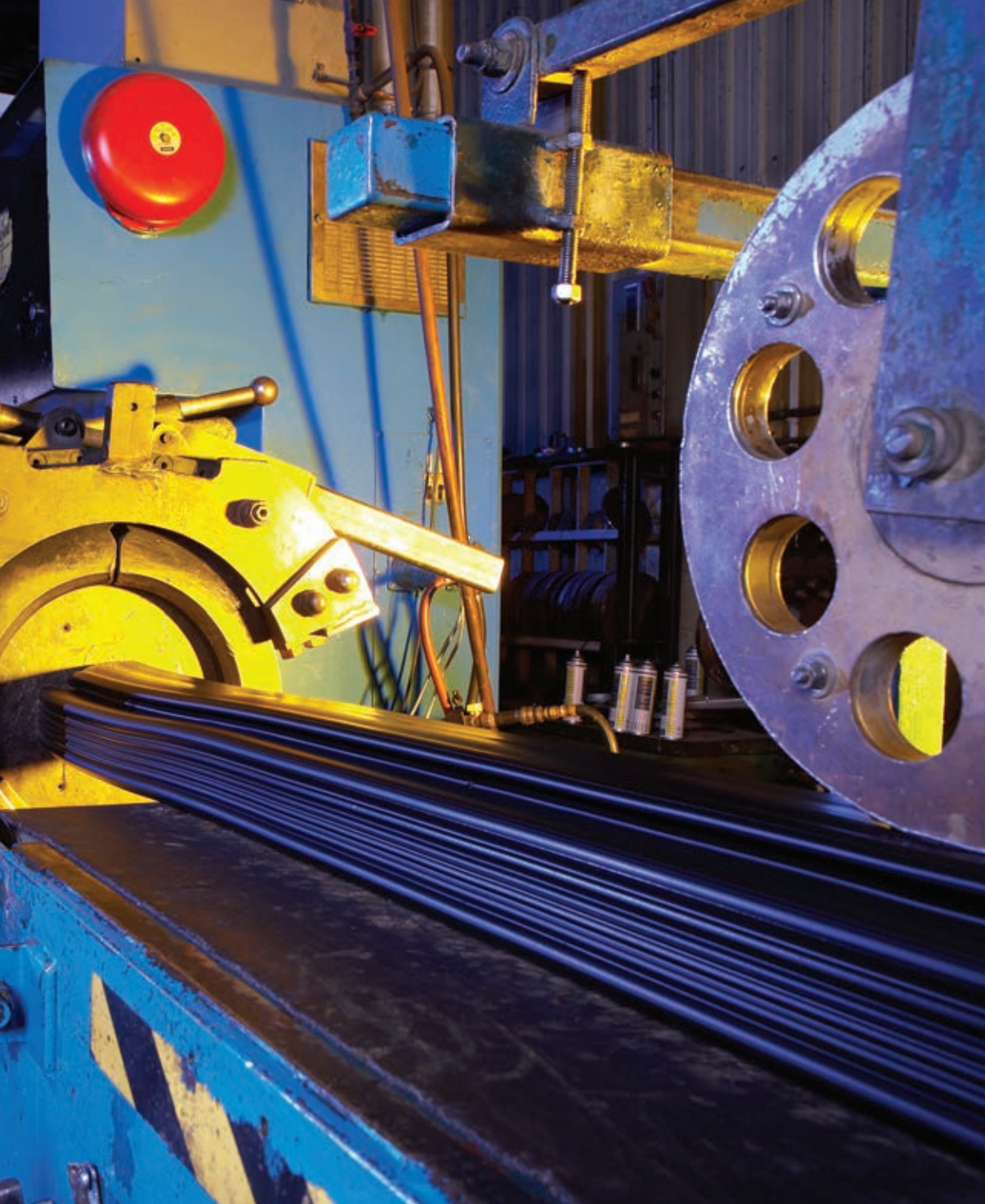
Polycorp's Epflex Railseal extrusion process.
