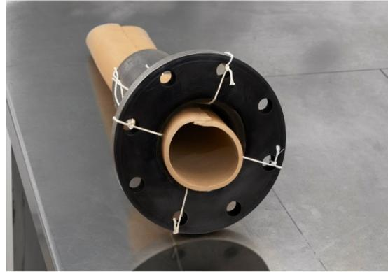
10, Expanding the tube against pipe wall
