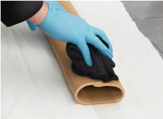
5, Applying solvent on the tube
