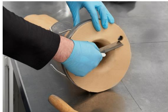
16, Cutting rubber out of bolt holes
