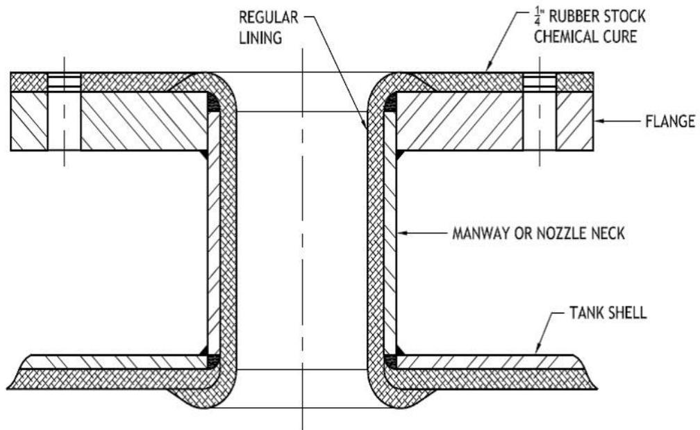
Fig. 10-5 Internal steam cure vessel flange detail for outlets
