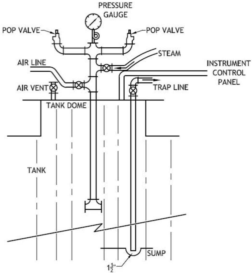
Fig. 10-1 Internal steam cure – tank with sump
