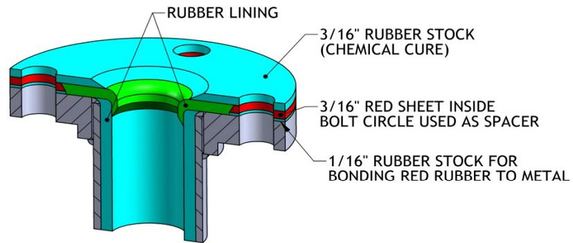
Fig. 10-3 Internal steam cure vessel - Flange detail for outlets
