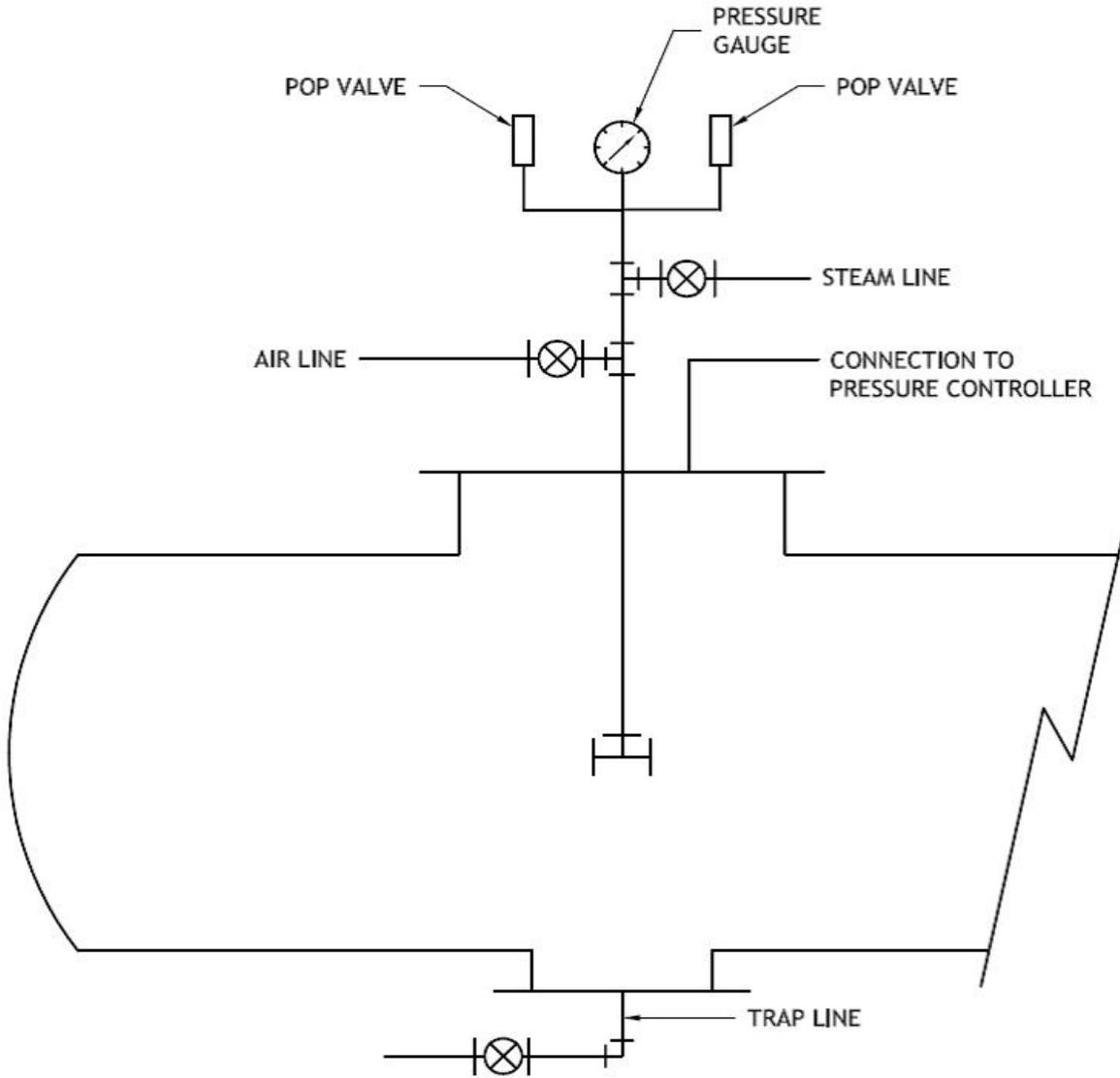
Fig. 10-2 Internal steam cure – tank without sump
