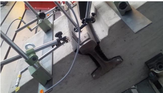
LRT tracks can now be constructed in the vicinity of studios, hospitals, and highly sensitive labs. At a fraction of the cost of a floating slab system, high vibration attenuation is achievable with Polycorp's resilient embedded system. It consists of rail boot, rail pad, steel tie, and all required hardware. Based on customers' needs, the system is tuned to deliver optimal performance with minimal cost.
