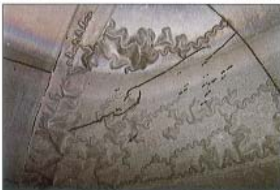
Wrinkled rubber lining on tank car head Courtesy of Jim Molnar, Union Tank Car
