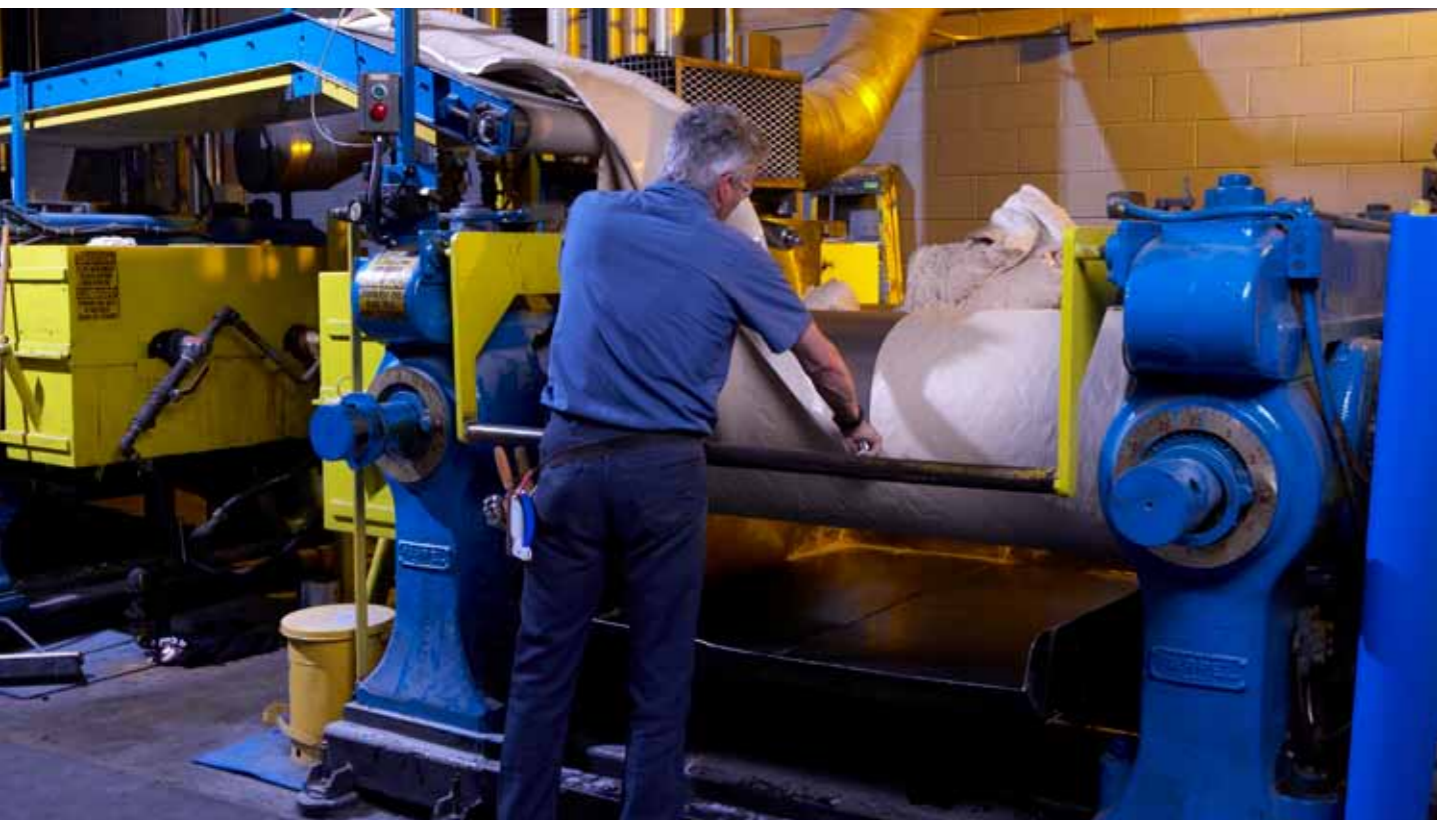
Protective linings warming mill
