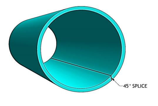
Fig. 8-1 Longitudinal skived butt splice
