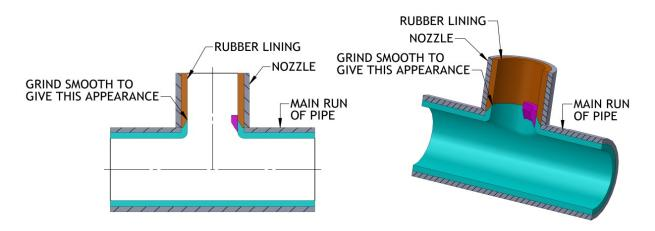
Fig. 8-5-2  $90^{\circ}$  nozzle details
