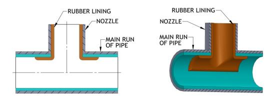
Fig. 8-5-1  $90^{\circ}$  nozzle details
