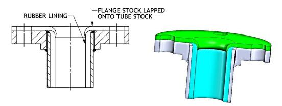
Fig. 8-3-2 Flange covering method (Flange stock lapped onto tube stock)
