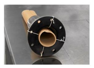
10, Expanding the tube against pipe wall
