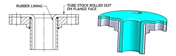
Fig. 8-2-2 Rubber lining to maintain thickness over the flange face (Tube stock rolled out on flange face)
