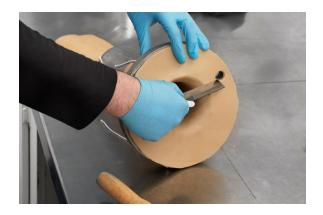
16, Cutting rubber out of bolt holes
