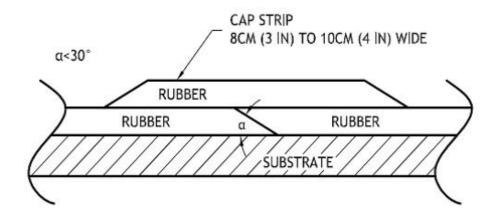
Fig. 6-3 Butt seam with strip
