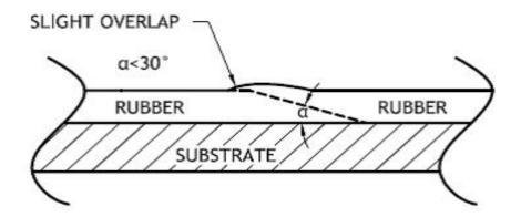
Fig. 6-4 Skive butt joint
