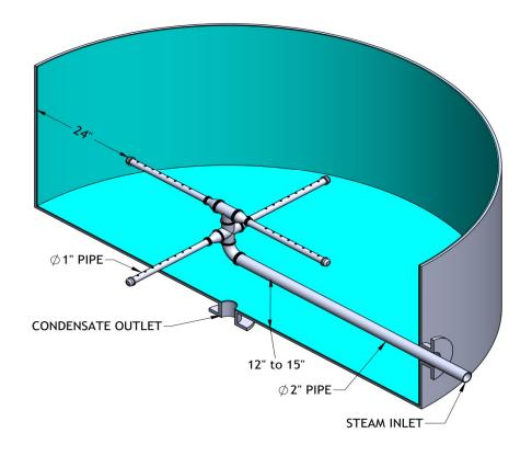
FIG. 10-7 TYPICAL EXHAUST STEAM PIPING SETUP
