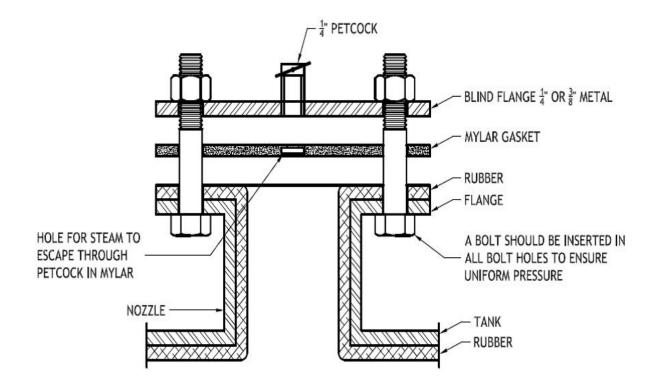
Fig. 10-6 Internal pressure steam cure – Flange assembly
