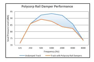
Open ballast track that is near residential areas can benefit from significant noise reduction without the need to dig up the tracks, add unsightly and costly sound walls, or add other invasive methods to control noise. Polycorp Dampers can also be easily added or removed without damaging the existing rail.
